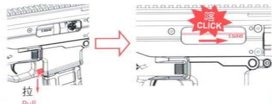
伸縮托操作 Operate the Telescoping Stock.
