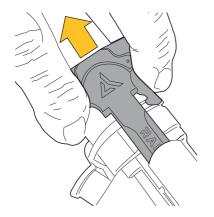
To open the chamber of the Model 1 gun, pull back on the charging handle.
