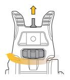
The front sight features the ability to adjust the sight post according to the elevation. Rotate the dial clockwise to raise and counter-clockwise to depress the post.
