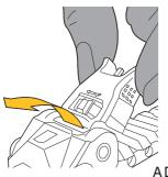
To engage the EPBUIS Front Sight upright, simply lift the sight by the textural plains on the sides to the ready position.
