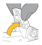
To engage the EPBUIS Rear Sight upright, simply lift the sight by the textural plains on the sides to the ready position.
