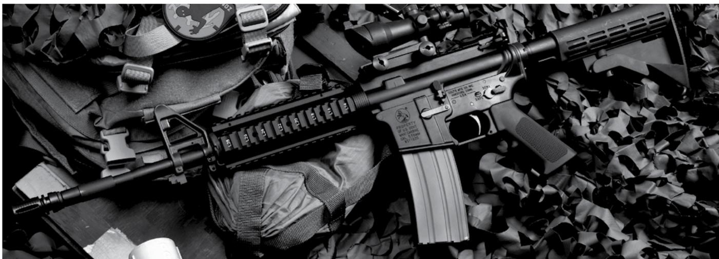
The M4 carbine is a family of firearms tracing its lineage back to earlier carbine versions of the M16, all based on the original AR-15 designed by Eugene Stoner and made by ArmaLite. It is a shorter and lighter version of the M16A2 assault rifle, with 80% parts commonality.
